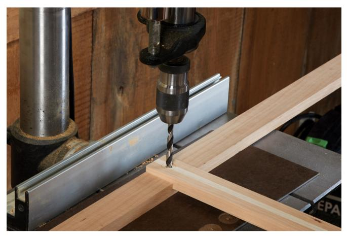
The stability of the drill press makes it easier to bore accurate holes than with a handheld drill.
