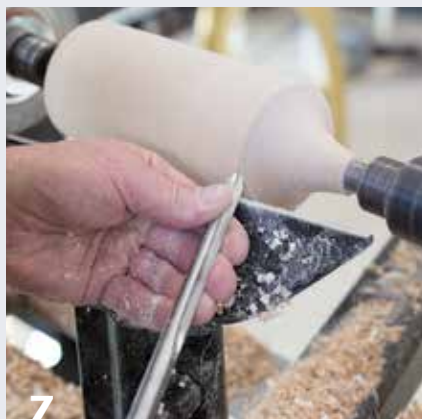
Cutting the left side of a cove illustrates the combination of the cutting arcs. Vertically, the tool handle moves upward; laterally, to the left; and rotationally, counterclockwise, with the flute twisting from 3 o'clock to 12 o'clock.
