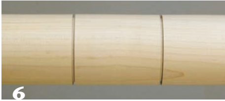
6 Maple: The first section is finished to 80 grit and the other two sections were finished with P80.
