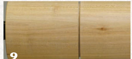
9 Cherry: At this viewing angle, no scratches are visible. Scratches become obvious when viewed at an angle, as in Photo 12.
