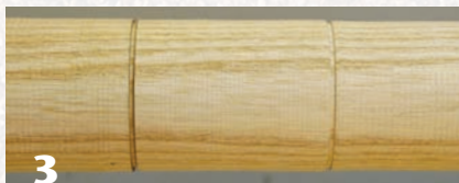
3 Ash cylinder prepared by scraping with a dull bowl gouge to produce torn grain and tool marks.
