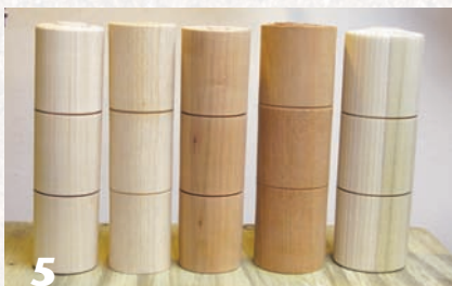
5 The various woods used, left to right: Maple, ash, cherry, mahogany, yellow poplar. The top section of each cylinder has been finished with Method 1 & 2-US to 320 grit. The middle sections are all finished with Method 1-EU to P400 grit. The bottom sections are all finished with Method 2-EU to P400 grit. Method 2-EU included grits P100 and P150, which were not used in any of the other sections.
