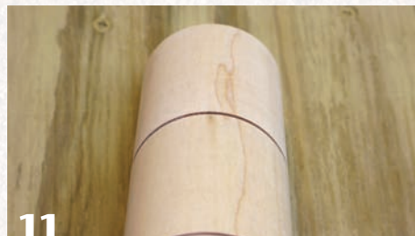
11 Maple: The same cylinder in Photo 8, but viewed at an angle to reveal scratches.
