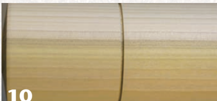
10 Poplar: The apparently smooth finish actually has abrasive scratches, which become noticeable when viewed at an angle, as in Photo 13.
