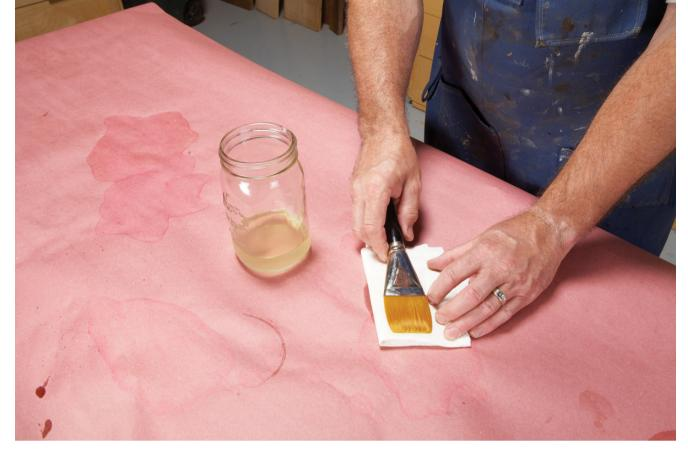
Pull the brush across a folded paper towel or rag to remove the excess alcohol. Form the bristles so they dry in their proper shape. The brush will dry stiff from the shellac left in the brush. To use again, soak brush in alcohol for a few minutes
