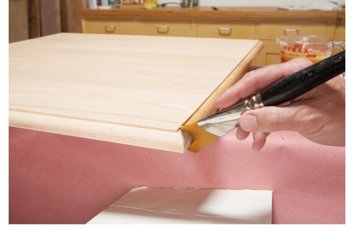
Come back to finish the bare spot where you started the stroke. Think of your brush as an airplane. Land the brush near the unfinished end and then lift off right at the edge to avoid snapping the bristles over the edge. Lifting off prevents pools of shellac from being left at the edge and turning into drips.
