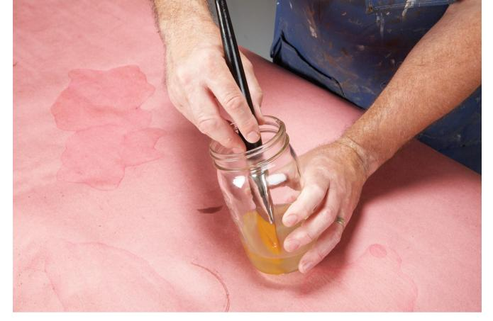
When the brushing is over, cleaning your brush is a breeze. Just swish it around in a container with clean denatured alcohol. This will clean out most of the shellac from the brush. Unlike varnish or water-based finishes, it okay to leave some residue in the brush.
