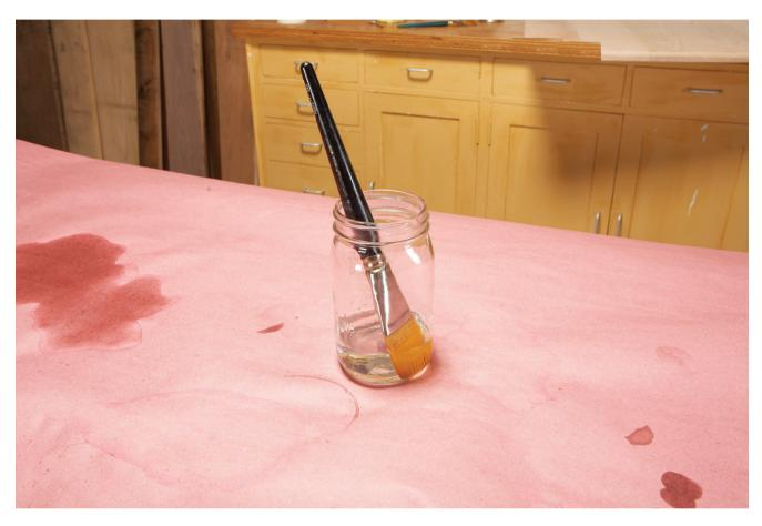
Charge the brush by soaking it in denatured alcohol for a few minutes before use. This helps the shellac flow better from the brush.
