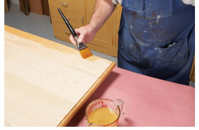
A different brushing technique is used on the top surface. Instead of a long and slow stroke, use short fast strokes. Land the loaded brush in a dry area and with rapid back and forth strokes work the shellac back into the wet area. Aim for a thin, even layer of shellac.
