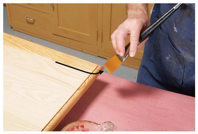
Finish the stroke at the edge. Lift the brush as it passes over the edge just like an airplane taking off. This prevents the brush from pushing shellac
