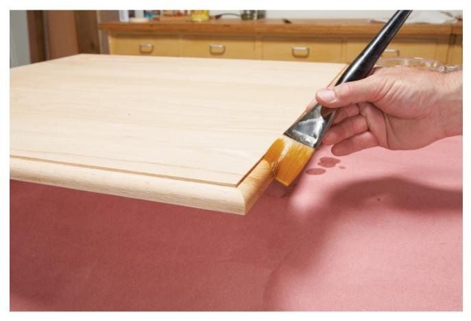
Shellac the edges first. Start the brush stroke an inch or two from the end. Move the brush slowly to lay down a long, consistent wet layer of shellac. Nestle the edge of the brush in the fillet to keep excess shellac from accumulating and running when your back is turned.
