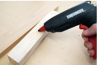
Once your wood glue is applied add a squirt of hot glue in the gaps of wood glue. Before the hot glue has a chance to set, join the wood pieces together and hold in place for a few seconds. The hot glue bonds the two pieces together with enough strength to keep working, and holding the wood in place until the wood glue can take hold and make a stronger bond.
