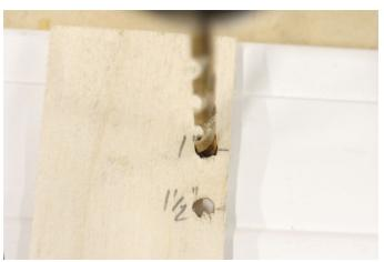
Taking this concept further a story stick can also be used from drilling holes a consistent distance from an edge. Make a story stick as usual, but this time drill an opening at the measured mark. Now your story stick can be used as a drill guide.
