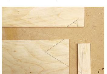
Whether you've got boards laminated together in a particular orientation, or just multiple pieces that need to be in a specific place, the triangle registration mark is a great tool to use.
