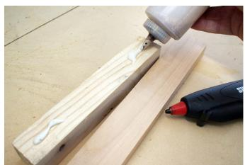
Plug in your hot glue gun and let it come to temperature before applying any wood glue. Once your hot glue is ready, apply wood glue as usual but leave small gaps every so often in the piece to be glued.
